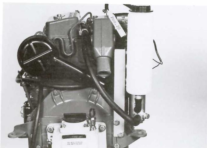
3. Montera värmeväxlarpaketet med originalbultarna till motorfästet. Loosen and remove the two upper M 10 Bolts B on the starboard engine mount bracket using the M 17 wrench. (see picture). Assemble the heatexchanger package to the engine mount using these two bolts. (see picture).
